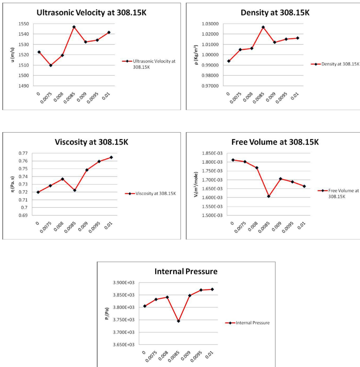
Fig 3: ultrasonic velocity, density, viscosity, free volume and Internal Pressure for aqueous L-Glutamic Acid at 308.15K
