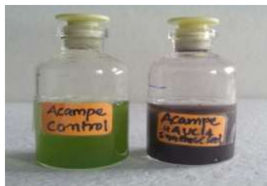
Fig.2. Acampe praemorsa leaves extract as control and bio reduction of gold nanoparticles as ruby red colour.
