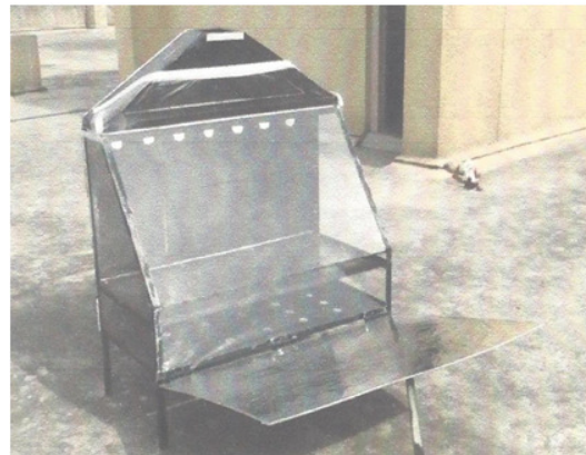
Figure. 2 Solar cabinet dryer along with reflector and chimney.
