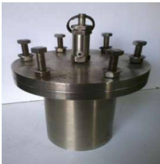
Fig-2: Autoclave used for Hydrothermal Synthesis
