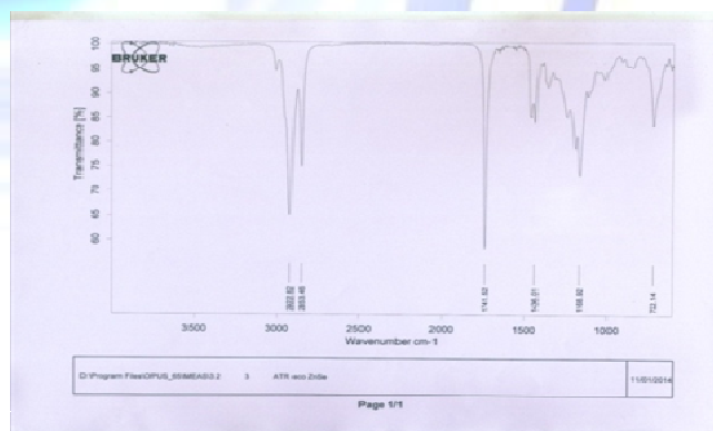
Fig.3: FTIR spectrum of biodiesel prepared from cotton seed oil.
