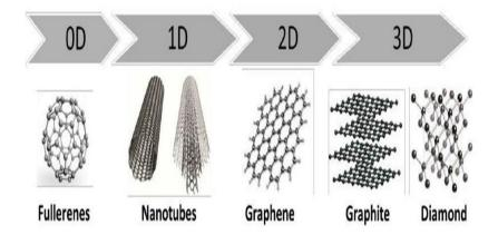
Figure 1:types of carbon based materials.  $\odot$  Source by, @phdthesis{phdthesis, author = {Srivatsa, Thushar}, year = {2017}, month = {08},title = {Graphene Based surface coatings on ceramic membranes for water desalination}
