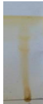
Figure. 3. Water extract (chloroform: methanol, 3:7). Developer-Iodine for TLC plates.
