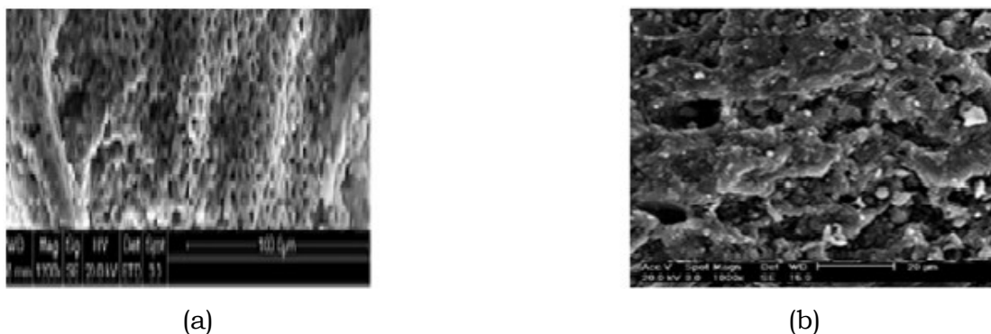
Fig. 4 (a) SEM of Pure 2-HABT(II) (b) SEM of GO-TiO 2 – 2-HABT photocatalyst
