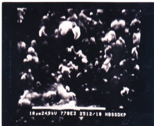
Fig 2 Scanning Electron microscopy as deposited CdO on glass substrate at, 300°C sprayed
