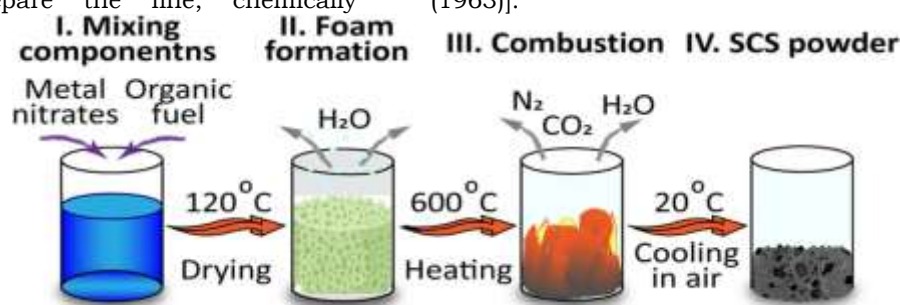
Fig.1.1 Schematic representation of solution combustion method
