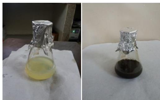
Fig 2:- Color change of Moringa oleifera plant extract before and after addition of AgNO3
