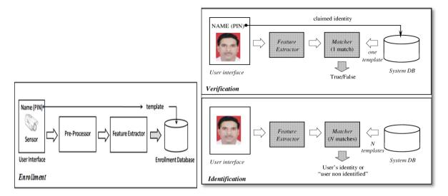
Fig. 1: Block diagram of a biometric system [1].
